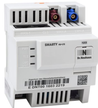
Figure 3: SMARTY IQ-LTE casing and external interfaces
