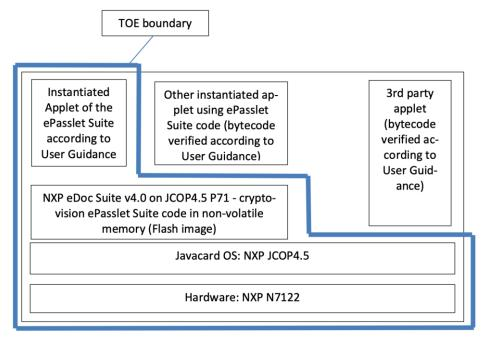
The whole applet code resides in the Flash memory; the applets providing these different configurations are instantiated into Flash memory. Multiple configurations (and hence support for different applications) can be present at the same time by instantiating multiple applets with their distinct configurations.
