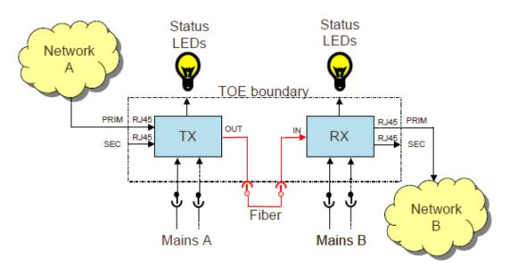
The subsystem TX contains a laser LED that converts electronic signals to light. The subsystem RX contains a photoelectric cell that can sense light and convert it to electronic signals. The fiber-optic cable allows light to move from the TX to the RX.
